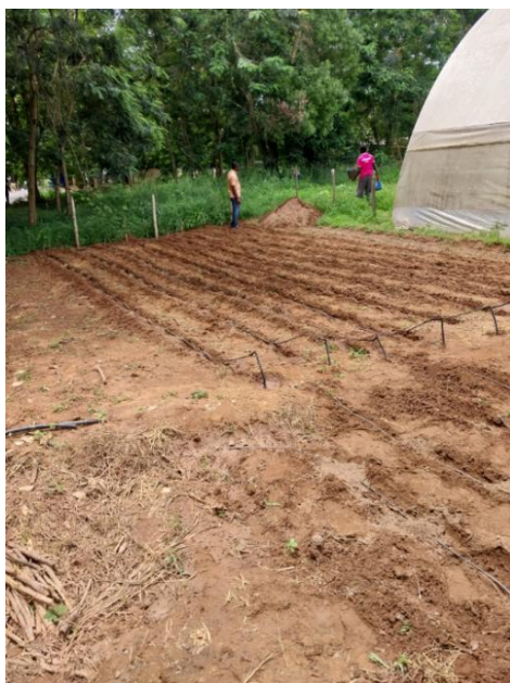
Figure 1. The experimental field showing dug trenches for installing the SLECI emitters (left), and sections of the CSDI treatment (right)
